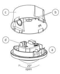
Turn the sensor unit (a) by about 20° counterclockwise, up to te snap-in point. Remove the sensor unit. Break out the required cable passages (b). Mount the surface-mounted housing (c) via the provided fastening holes to the ceiling. Perform the wiring (d). Put on the sensor unit (a).
