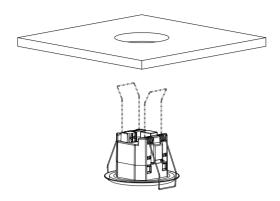
Installation in false ceilings for ceiling thicknesses of 0.5 mm to 3 cm. The diameter of the ceiling cutout must be between 62 mm and 70 mm.
